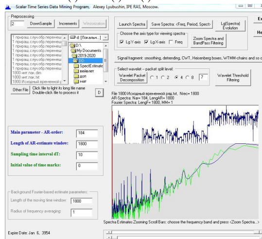
Fig.1 Maximum entropy estimate and «background» Fourier estimate of the source series
